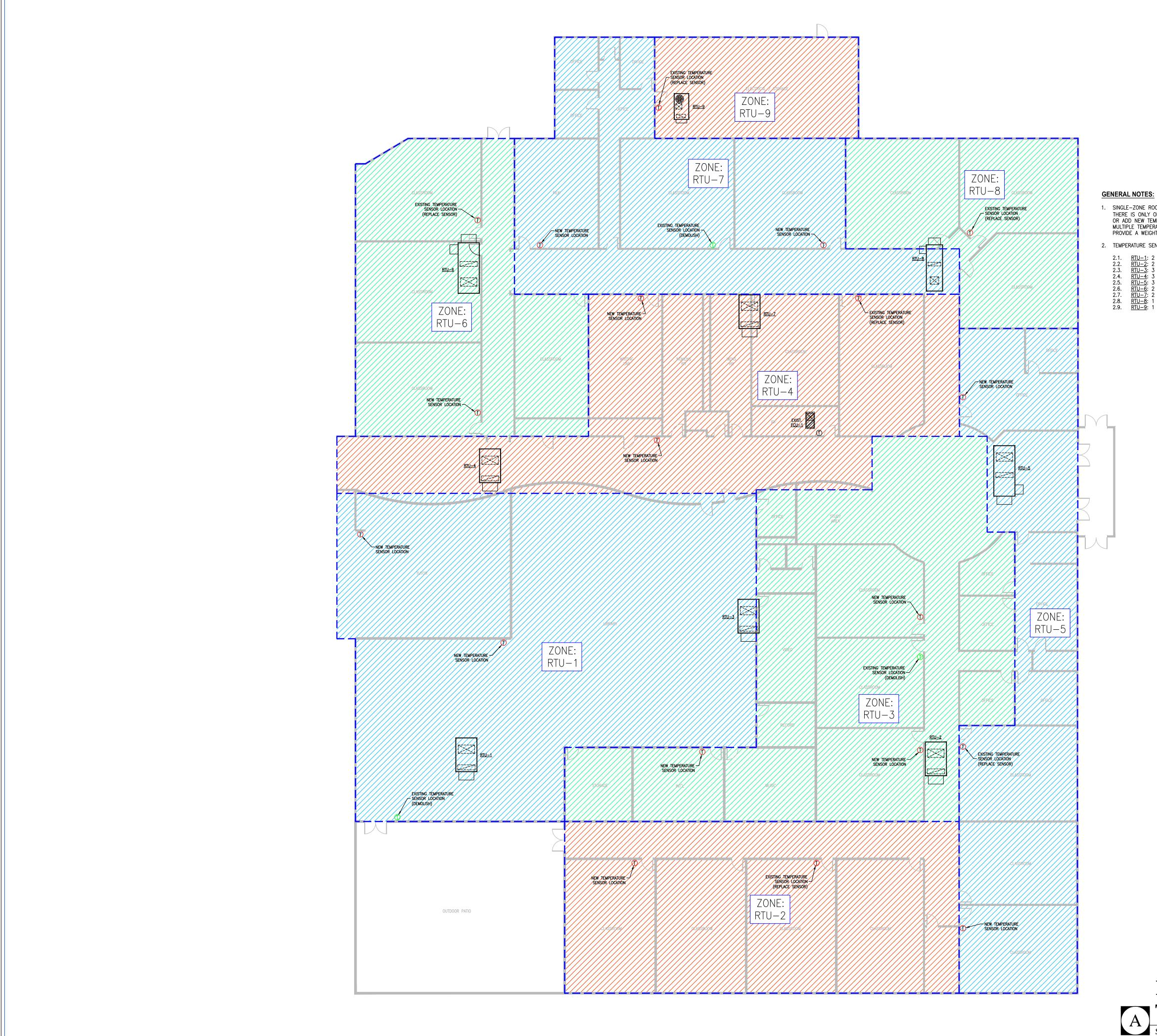
1. SINGLE-ZONE ROOFTOP UNITS SERVE MULTIPLE ROOMS. RECORD DRAWINGS INDICATE THAT THERE IS ONLY ONE TEMPERATURE SENSOR PER ZONE. REMOVE, REPLACE / RELOCATE, OR ADD NEW TEMPERATURE SENSORS AS INDICATED ON THE DRAWING. FOR ZONES WITH MULTIPLE TEMPERATURE SENSORS, AVERAGE THE SENSOR TEMPERATURES FOR RTU CONTROL. PROVIDE A WEIGHTED AVERAGE ALGORITHM TO ALLOW ADJUSTMENT OF SENSOR PRIORITY.
